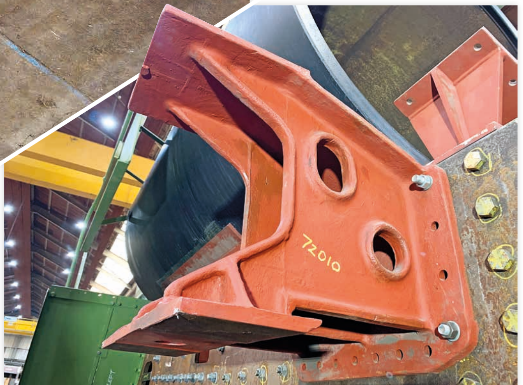
▼ With the main components of the 'Clan' frames now brought together, work is progressing on adding other items, such as this slide valve bracket.
