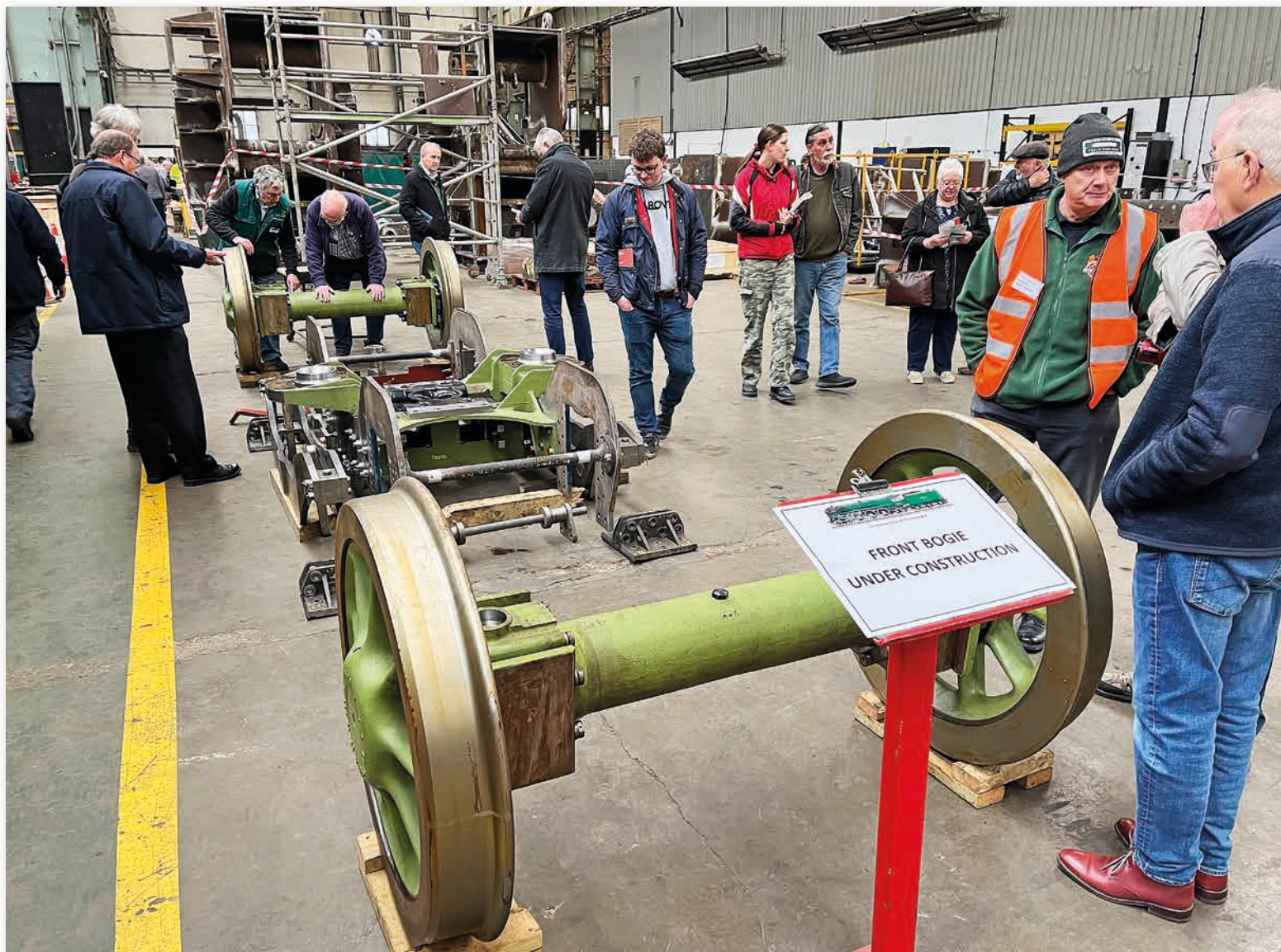
The front bogie for Hengist under construction. The TRACKSIDE-supported open day attracted a wide variety of people, including many locals who were keen to see what goes on in the vast buildings. Paul Appleton
